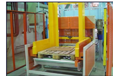
EMPTY PALLET MAGAZINE & DISPENSER
