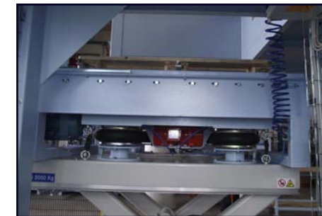
VIBRATOR TO SETTLE THE PRODUCT INSIDE THE BAG
