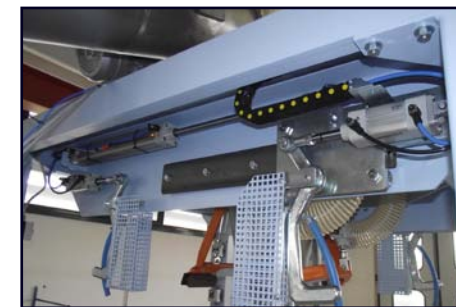
MOVABLE HOOKS TO FIX THE EMPTY BAG FROM ONE POSITION
