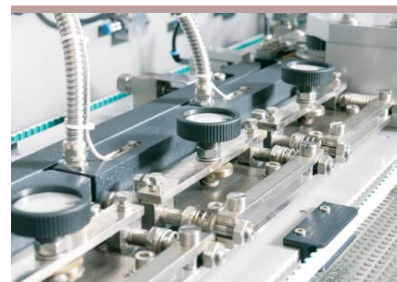
Sealing tape application
