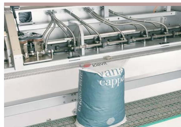
Heating section for inner-liner sealing
